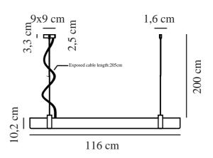
Voltage (V): 220-240 Volt IP degree: IP20 Maximum bulb wattage (W): 28W Class (Class 1, Class 2, Class 3): Class 2 (Double isolated) Socket type: LED Module Dimmerable: True
