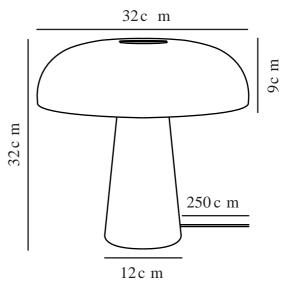
Voltage (V): 220-240 Volt IP degree: IP20
