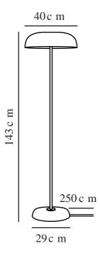
IP degree: IP20 Maximum bulb wattage (W): 3x25 Class (Class 1, Class 2, Class 3): Class 2 (Double isolated)
