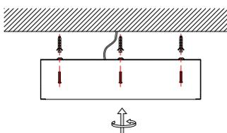
Drill holes, Apply plastic anchors & screws
