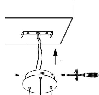
Fix the luminaire into place by tying up the side screws
