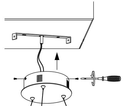
Fix the luminaire into place
