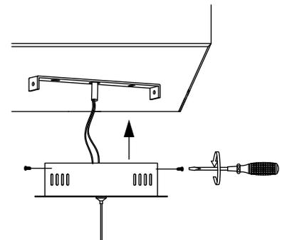
Fix the luminaire into place by tying up the side screws
