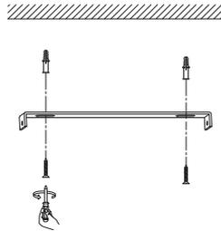
Drill holes Apply Plastic Anchors
