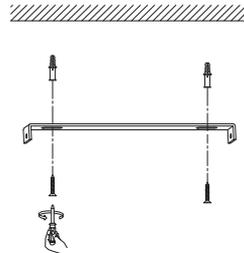
Drill holes Apply Plastic Anchors
